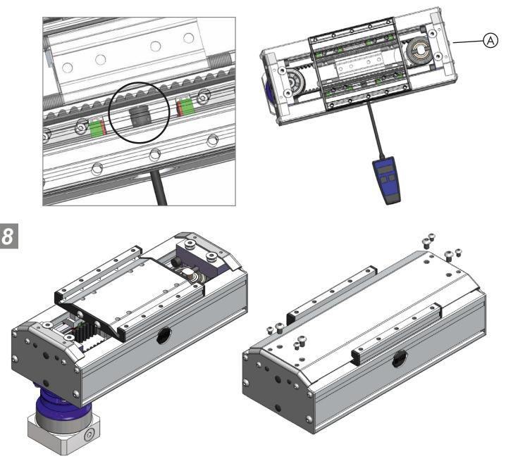
After the mounting procedure is completed, the cover plate can be re-mounted following the steps in reverse order. Ensure that the inner screws are tightened first. Finally tighten the small outer screws.
