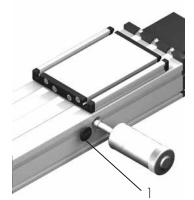
Lubrication is effected by an oiled felt insert. The felt can be re-oiled through lubrication nipples attached laterally to the ends of the roller packs.
